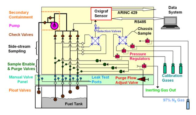
The above system process schematic shows the O2N2 analyzer in relation to the float valves in the fuel tanks, the purge and calibration gasses and flows, and the control and data system. Communications to the control and data system are through RS-232/485 links and an ARINC-429 interface is provided to communicate with customer furnished data monitoring and recording systems.
